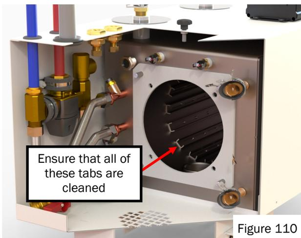
11. Remove the combustion chamber to gain access to the heat exchanger as shown above.
